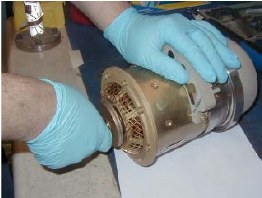
Figure 3 Radial Measurement Check
