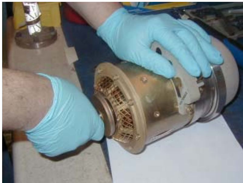
Figure 3 Radial Measurement Check
